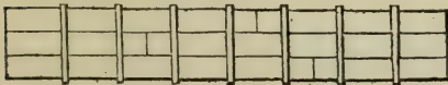
Fig. 85—Represents a solid built beam of three courses, the pieces of each course breaking joints and confined by iron hoops.
